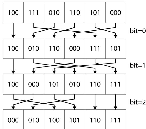
FIGURE 5.2: Radix sort loops over the bits of the key starting at the least-significant bit. All keys with a 0 in the bit are placed before keys with a 1. The process is repeated for each bit resulting in a sorted list.
