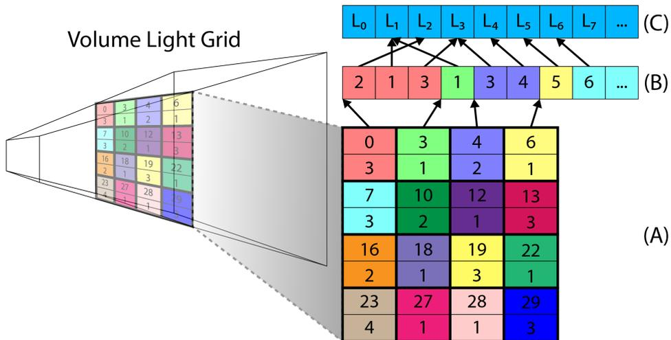
FIGURE 8.3: A single slice of the volume light grid (A). The light grid stores the light count and an offset into the light index list (B). The light index list stores the index of the light source in the light list (C).
