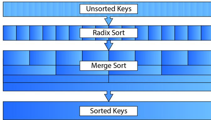
FIGURE 5.1: In order to sort the keys, a hybrid sorting approach is used. The unsorted keys are first sorted into chunks of 256 keys using a parallel radix sort. A merge sort is repeatedly applied to the sorted chunks to produce the final sorted list.
