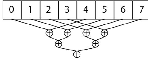
FIGURE 4.3: Interleaved log-step reduction. Accessing both global and shared memory is optimized.
