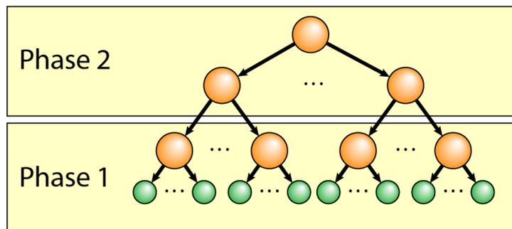
FIGURE 7.2: In the first phase of the BVH construction, the AABB of the child nodes of the last level of the BVH tree are computed from the sorted scene primitives. In the second phase of the BVH construction, the upper nodes are computed.
