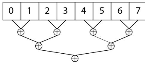
FIGURE 4.2: Pair-wise log-step reduction. This method does not make optimal use of memory access patterns in GPU memory.
