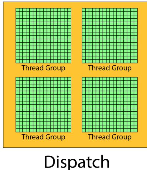
FIGURE 3.1: The dispatch consists of thread groups. Each thread group consists of a number of threads. This image shows a two-dimensional dispatch but the dispatch can be either one, two, or three-dimensional.
