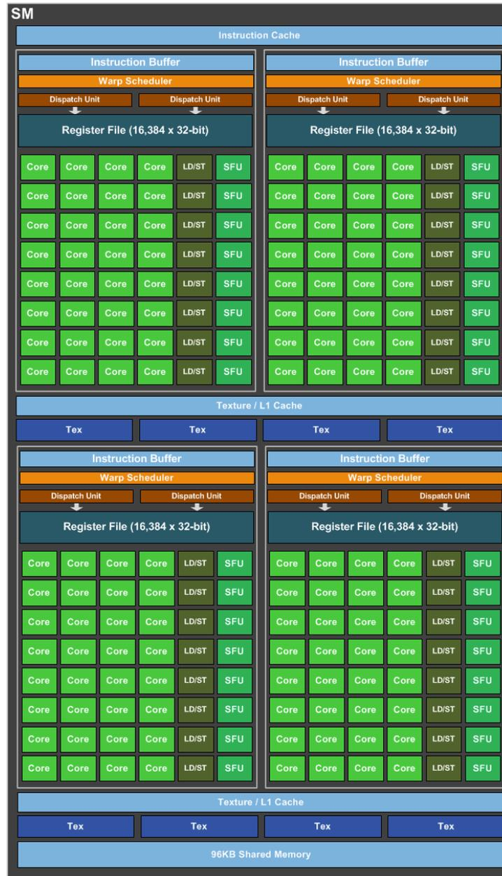
FIGURE 3.2: Pascal GP104 Streaming Multiprocessor architecture.
