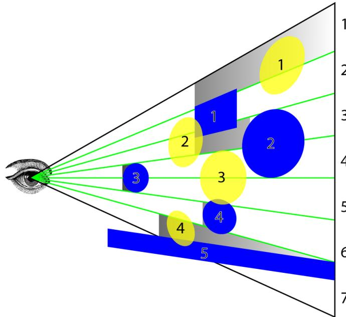
FIGURE 2.13: The blue objects in the image represent opaque scene objects. The yellow spheres represent light sources, and the gray shaded areas represent the depth range of the tile's view space frustum. Light 1 is incorrectly included in the frustum for Object 1 because the object partially covers the first tile creating a depth discontinuity in the tile (Oosten, 2015).
