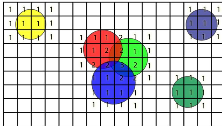
FIGURE 2.11: Lights overlapping tiles in the tile grid.
