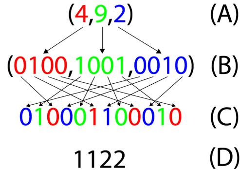
FIGURE 6.2: The integer representation of a coordinate in 3D space (A); The 4-bit binary representation of the coordinates (B); The result of interleaving the bits of the coordinate components (C); The resulting 12-bit Morton code in decimal representation (D).
