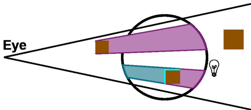
FIGURE 2.9: Find pixels inside the light volume and compute shading.
