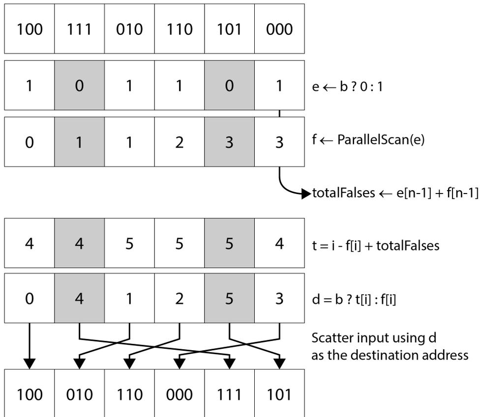
FIGURE 5.3: The radix sort algorithm applied to the least significant bit of the input.
