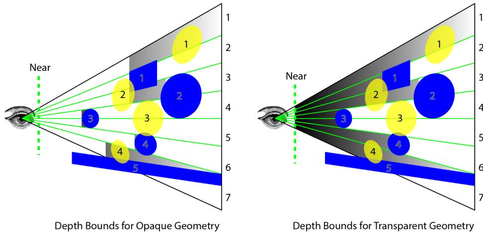
FIGURE 2.14: The culling frustum for opaque geometry can be derived from the minimum and maximum depth bounds within the tile (left). The culling frustum for transparent geometry uses the maximum depth value and the camera's near clipping plane (right). (Oosten, 2015).
