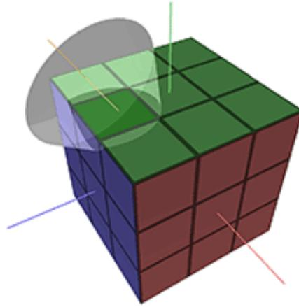
FIGURE 2.16: Normals are quantized to a 2D grid mapped over a cube (Olsson, Billeter, and Assarsson, 2012).
