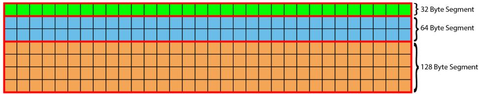
FIGURE 3.3: Global memory segments are 32 B for 1 B words, 64 B for 2 B words, and 128 B for 4, 8, and 16 B words.
