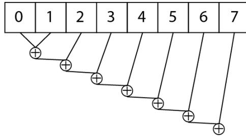
FIGURE 4.1: Serial reduction applied over an array of eight values.
