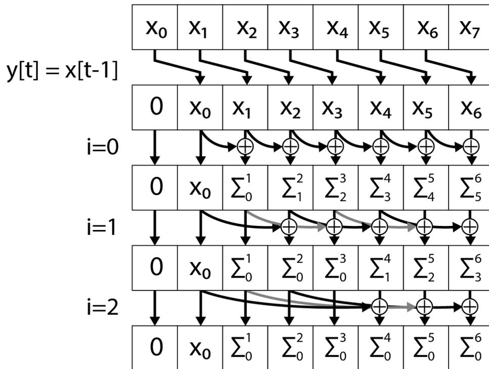
FIGURE 4.5: Parallel scan. For each iteration  $i$  of the parallel scan, each thread  $t$  larger than  $2^i$  computes  $x[t] \oplus x[t - 2^i]$  and stores the result at index  $t$ .
