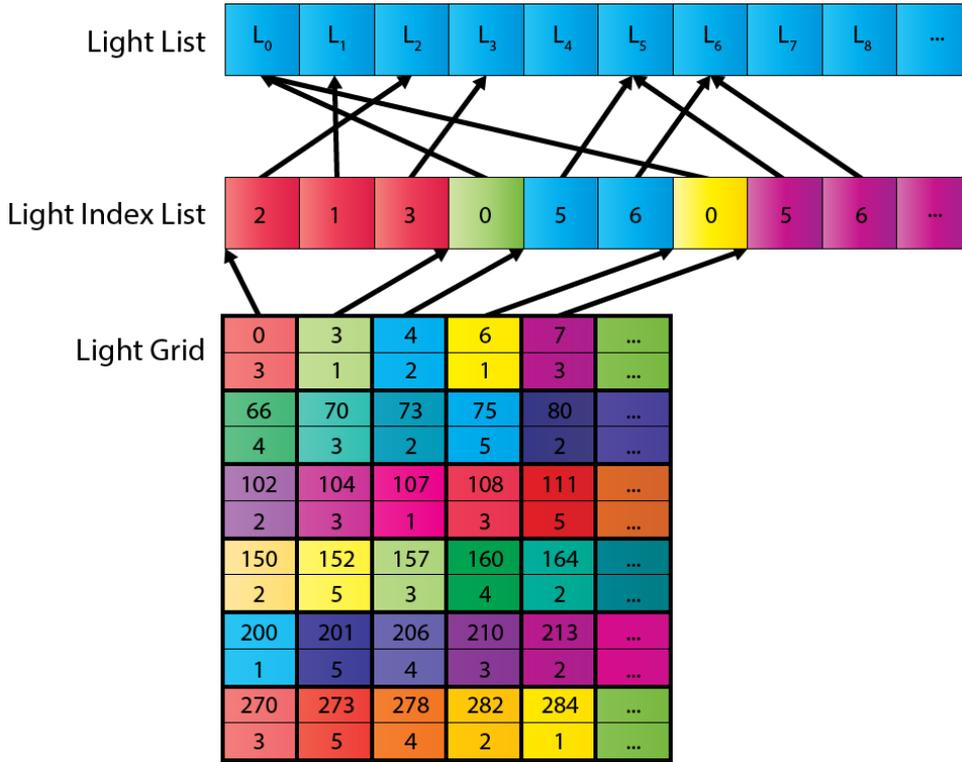
FIGURE 2.12: The data structures that are used to store the per tile light lists. The *Light Grid* stores the offset and the number of lights in the global *Light Index List* for each tile.
