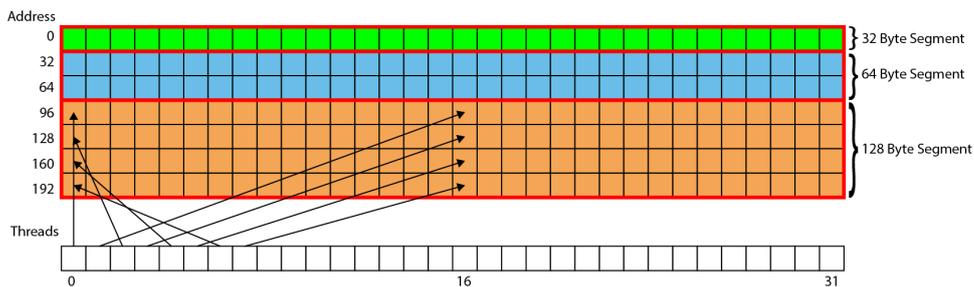
FIGURE 3.4: Each thread in a warp accesses a 16 B (4-component floating-point value) from global memory. This will result in 4 128 B memory transactions.
