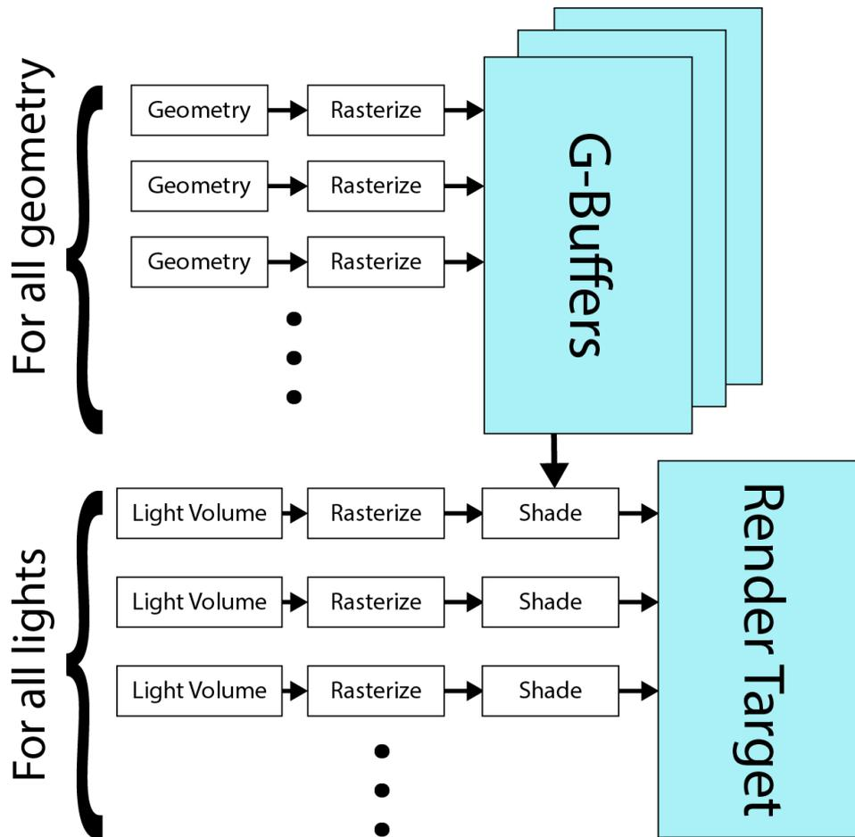
FIGURE 2.2: Deferred shading operates in two passes: Geometry pass and the lighting pass.
