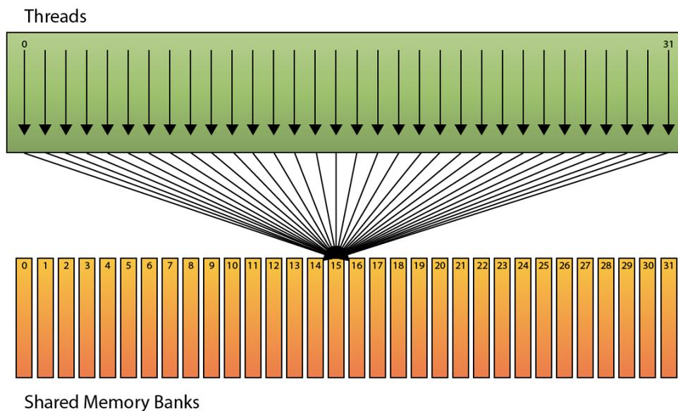
FIGURE 3.6: If every thread in a warp accesses the same address of a shared memory bank then the value is broadcast to all threads. In this case, no bank conflict occurs and all reads can be performed simultaneously (Oosten, 2011).
