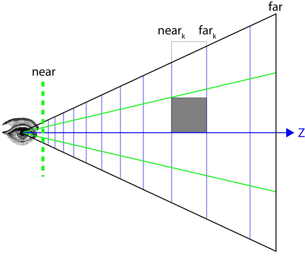
FIGURE 2.15: The cluster grid uses exponential spacing in the depth in order to keep the clusters as cubic as possible.
