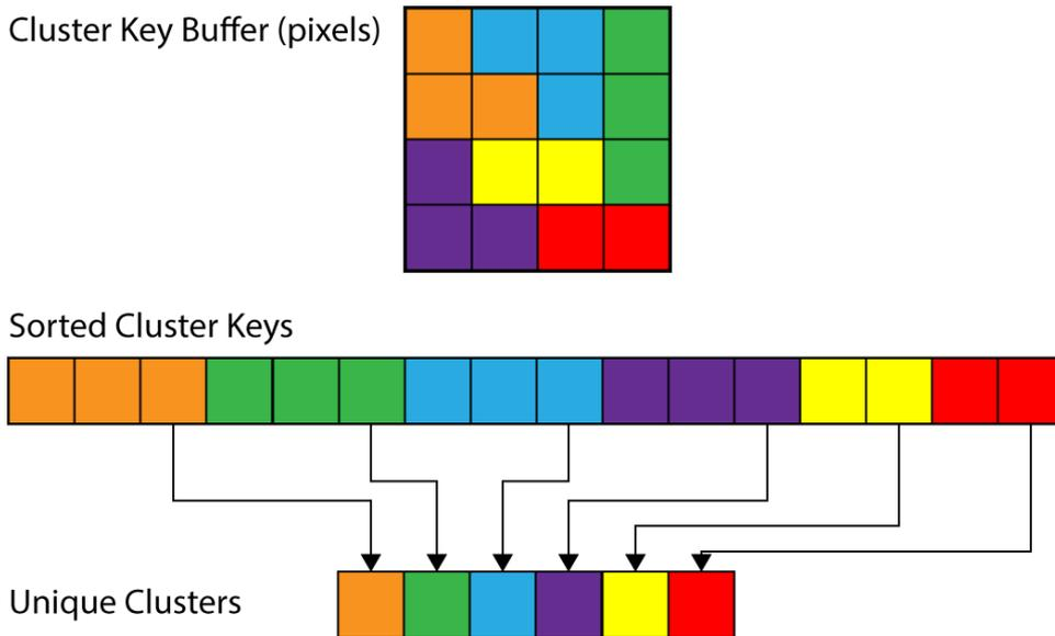
FIGURE 2.18: Unique Clusters: the cluster key buffer is sorted and compacted to find the unique clusters.
